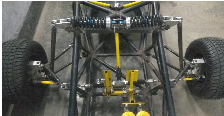
Fig. 8.1: The suspension system according to the design
